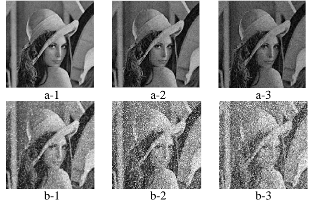
Fig. 12: The output of (a) stochastic and (b) conventional DWT with noise level of (1) 5%, (2) 10%, and (3) 15%.
