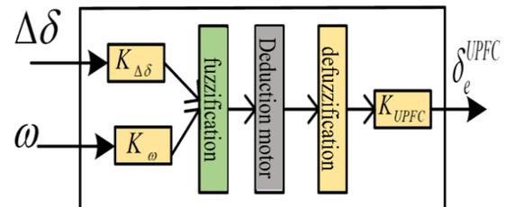
Fig. 6: Block diagram of the UPFC's fuzzy controller.
