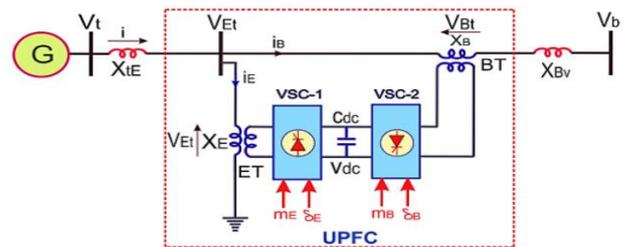
Fig. 3: A single-machine power system with a UPFC.
