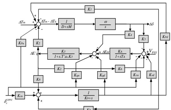
Fig. 4: Block diagram of the power system with a UPFC.
