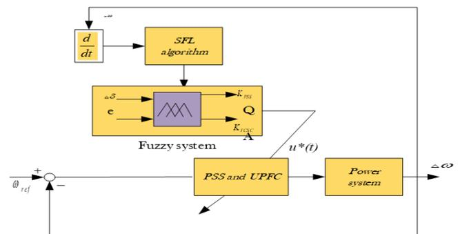
Fig. 1: Structure of the developed control design using a fuzzy controller.
