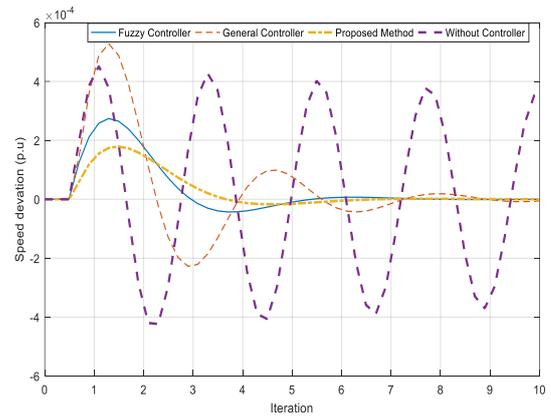
**Fig. 8:** Comparison of response of speed changes of three controllers for UPFC and PSS in 80% of the rated load.
